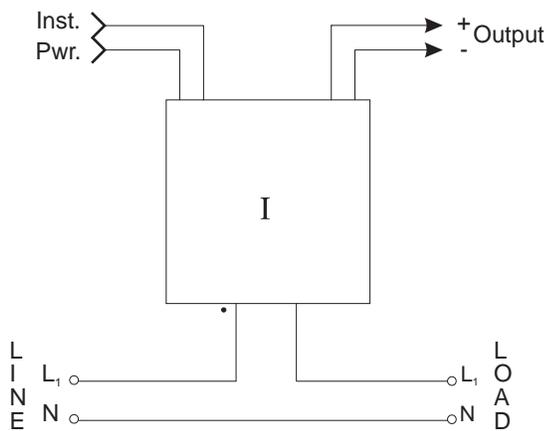
c) Current Transducer, Typical Installation, no Current Transformer
