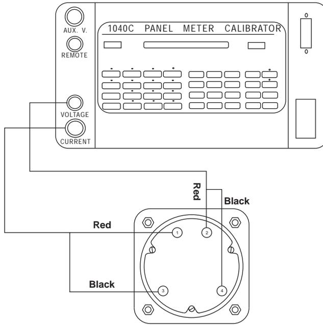
**SINGLE PHASE WATTMETER AND VARMETER**
