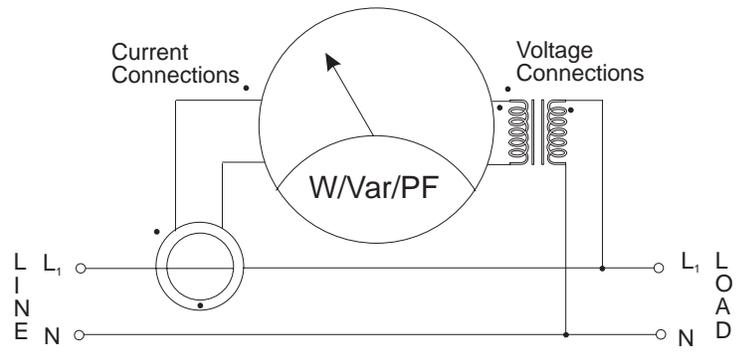
b) W/Var/PF Meter, Typical Installation, with Current and Potential Transformers
