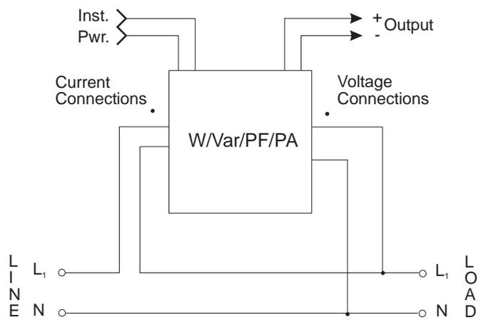
c) W/Var/PF Transducer, Typical Installation, no Current or Potential Transformers
