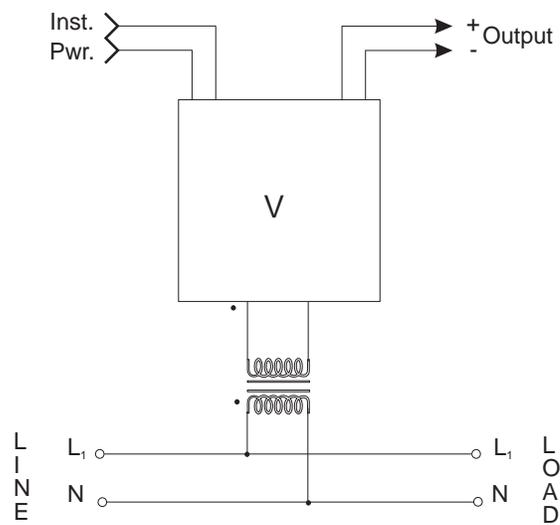
d) Voltage Transducer, Typical Installation, with Potential Transformer
