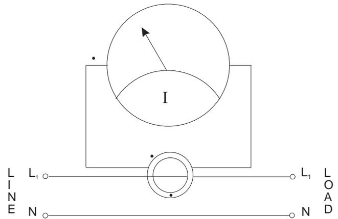
b) Current Meter, Typical Installation, with Current Transformer
