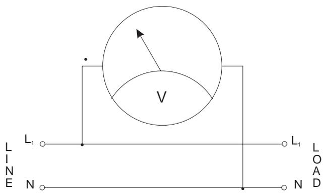
a) Voltmeter, Typical Installation, no Potential Transformer
