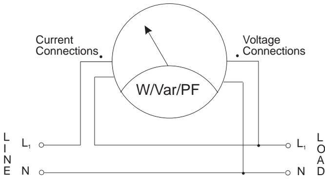
a) W/Var/PF Meter, Typical Installation, no Current or Potential Transformers
