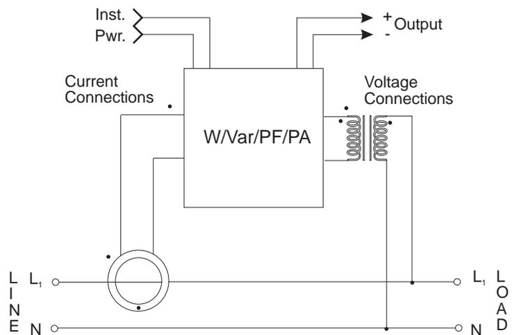
d) W/Var/PF/PA Transducer, Typical Installation, with Current and Potential Transformers
